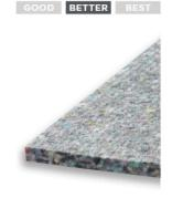
Style Num H8025 H8838 H8076 **Density** 8.0 lbs 8.0 lbs 8.0 lbs Thickness 1/4" 3/8" 7/16" 1/2" Roll Size 6' × 45' 6' × 45' 6'×45' 6'×45' yd2/Roll 30 30 30 30 FHA Class II Class II Class II Class II Certified Insulation R 0.91 R 1.37 R 1.82 Rating Recycled Yes Yes Yes Content Yes Yes Yes Yes Recyclable Cushion 15 year 15 year 15 year 15 year Warranty
